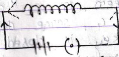
Let in a circuit, a inductor coil is connected in a circuit. When the switch is closed then the emf in circuit increases gradually from 0 to  $I$ , due to this an opposing emf is induced in the same coil which is shown by dotted arrow. ex:- choke coil.
