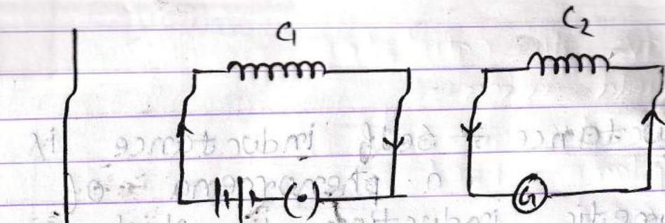
Let two circuits are arranged as shown in figure when switch is closed in  $C_1$  current rises from 0 to  $I$  and deflection in galvanometer of  $C_2$  can be seen, in  $C_2$  direction of emf is opposite to  $C_1$ , same deflection is observed when the key is closed.
