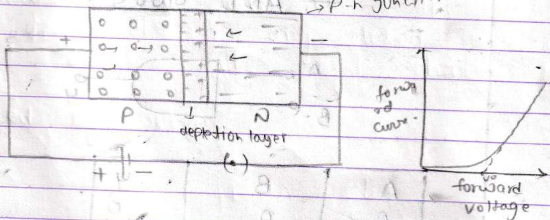
A p-n junction is said to be forward biased if p-part of the junction is connected to positive terminal and n part is connected to negative terminal. P-N junction diode carry current in forward bias.
